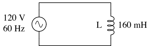
Figure 11.3: AC circuit with a purely reactive (inductive) load.
