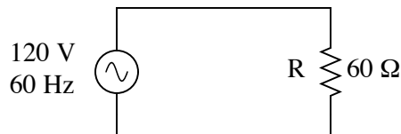
Figure 11.1: Ac source drives a purely resistive load.
